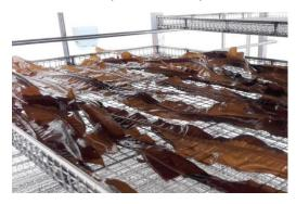
Our seaweed is dried within chambers containing dehumidifiers and fans to maintain strong airflow around the chamber. At the end of the cycle, the temperature is raised to around 40-45°C. All our seaweed is dried to below a water activity ( $A_w$ ) of 0.60, below which microorganisms cannot proliferate. Indeed, typically our seaweed is down to 0.30-0.45  $A_w$  when removed from the drying chambers.
